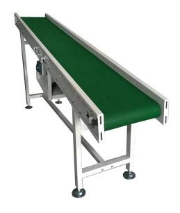
Belt conveyors are the most commonly used powered conveyors because they are the most versatile and the least expensive. Products are conveyed directly on the belt so both regular and irregular shaped objects, large or small, light and heavy, can be transported successfully.
