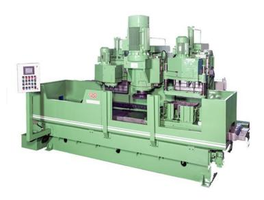
SPMs or Special Purpose Machines offer tremendous scope for volume production at investment and at low cost of production when compared to CNC SPM, machines. Special Purpose Machines is а high productivity with specially machine, designed tooling and fixture, dedicated for mass producing the same component day in and day out. A judicious combination of limit switches, sensors, logic controls, automatic job clamping etc is the essence of a SPM
